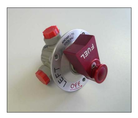
Andair Ltd. has issued a Service Alert for the Andair Fuel Selector Valves and Gascolators supplied with EF20/EF25 female fittings. Builders should inspect the stainless steel screws holding the female fittings to the fuel selector valve body to ensure they are tight and properly secured to prevent them from backing out. See the attached letter from Andair Ltd. for more information.
