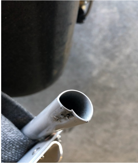
Typical damaged seat back tube, at the bottom.
