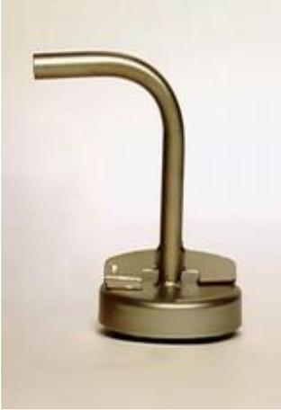
This photo of a fuel cap is for a Piper Cub with 180HP.
