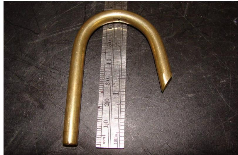
Above photos are from Zenith customers. Note the small hole in the gooseneck bend. Once installed properly, you can then seal the vent tubes that exit under the wings.
