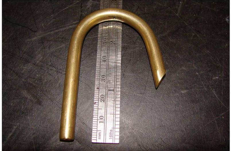
Above photos are from Zenith customers. Note the small hole in the gooseneck bend. Once installed properly, you can then seal the vent tubes that exit under the wings.
