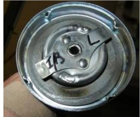
Above photos are from Zenith builders. Photo on the right shows the welding of the gooseneck tube and the plugging of the air vents in the cap.
