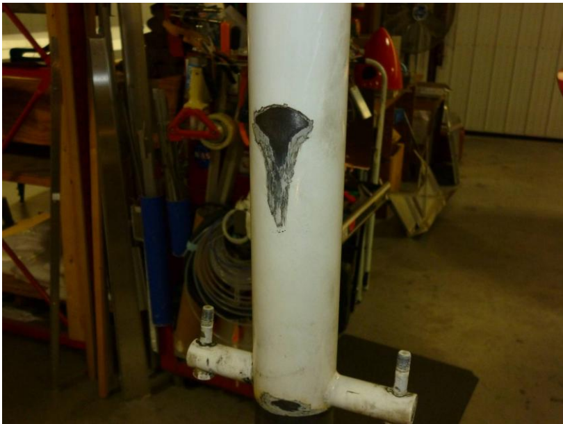
Photo shows the Nose Gear Strut wearing from the Bungee Pin.
