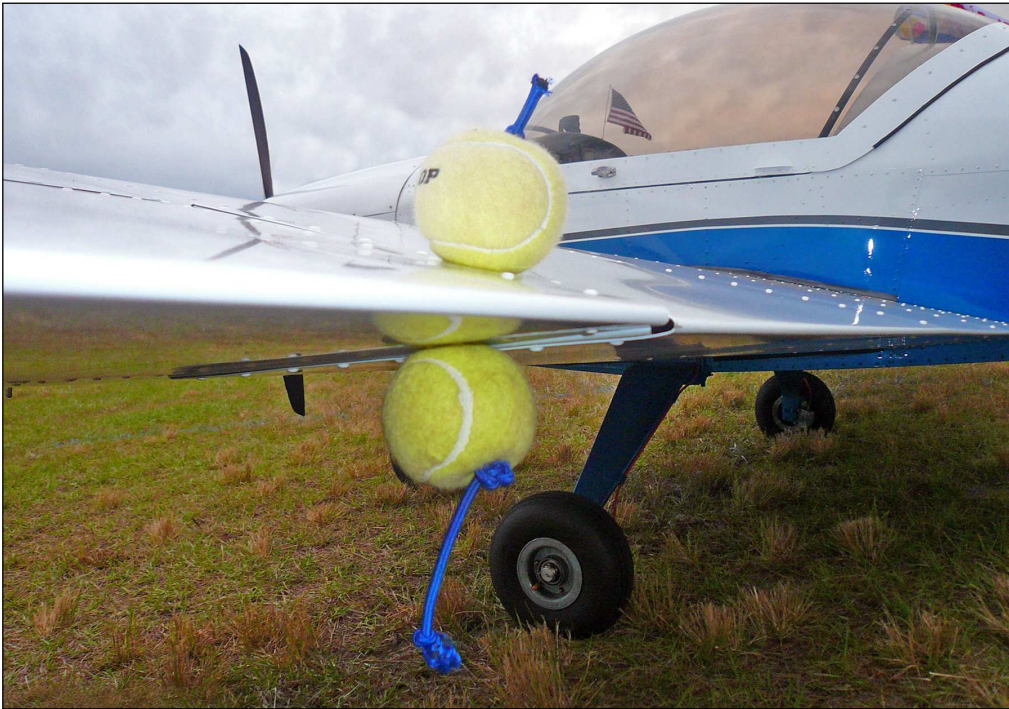
Above: Aileron control lock made from two tennis balls and a bungee cord.
